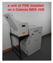
An internal film cassette is provided which is pre-loaded with exposed films ready for developing, the loaded cassette is then inserted into the **FDS** whereupon films are detected and the automatic loading can commence.
