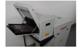
This operation is continuous until the last film is removed from the cassette. If required, urgently needed films can be added into the cassette by stopping and restarting the automatic operation. The functions of the FDS are continuously monitored to ensure any failure is detected and the operator informed.
